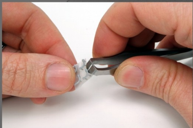
first of all cut of the part to the sprue with our STEEL CUT TWEZEER HDMU001
